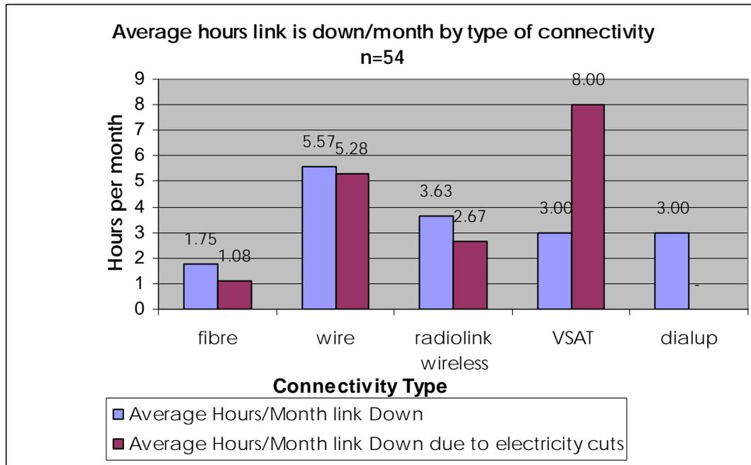
The results indicate that wired connections have a higher rate of failure, with 5.57 hours per month, than other links, with fibre having the lowest rate of failure of 1.75 hours per month. It appears that, where electricity cuts are a problem, VSAT and wire are affected most with 8 and 5.28 hours per month respectively. The implications of these findings are that VSAT and wire appear to be a more
